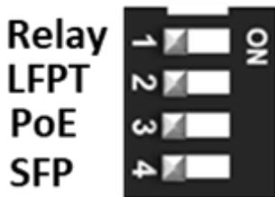
**\*Note:** There are four white buttons for DIP switch. Moving the white button up position, its setting is "ON". Moving the white button down position, its setting is "OFF".
