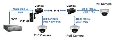
A total of 8 IP addresses can be accessed on a single cable run eliminating the need for network switches.
